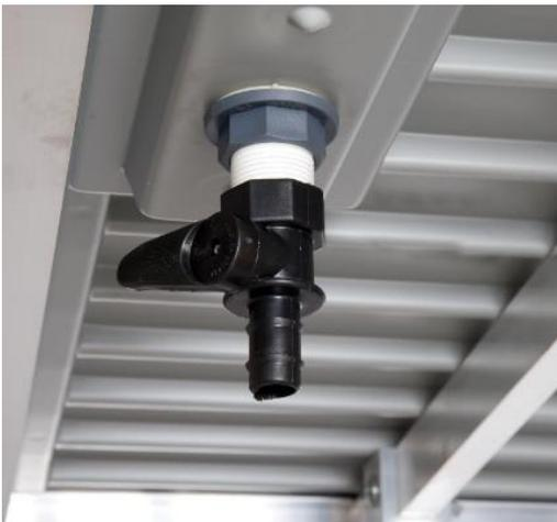
Minivalve threaded/barded 16x3/4" and tank adaptor with male threaded end G1 with clamping collar and EPDM flat gasket.
